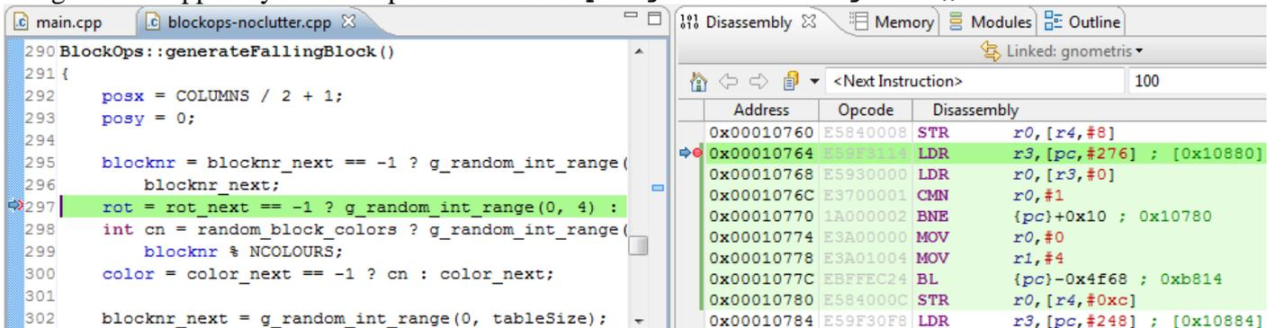
The current PC location is shown by an arrow (👉) in the left margin of both the source and **Disassembly** views and by the dark green highlighting. The light green highlighting in the **Disassembly** view shows all of the assembly instructions that correspond to the current source line.
