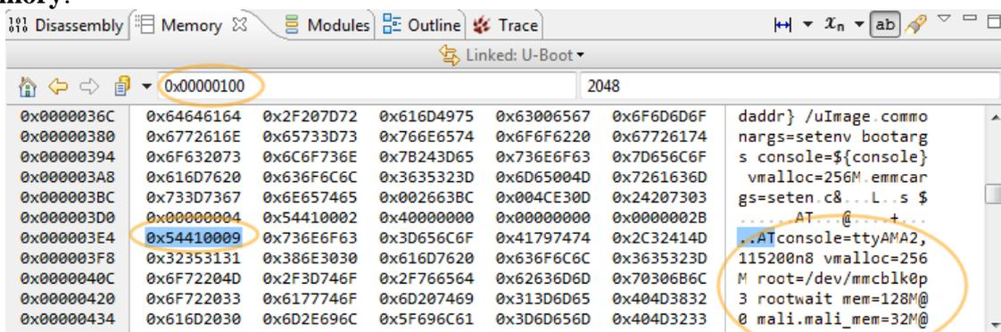
In the **Memory** view (you may need to scroll down) we can see the kernel command line string in the middle of the kernel parameters preceded by the tag value `0x54410009`: `console=ttyAMA2,115200n8 vmlloc=256M root=/dev/mmcblk0p3 rootwait`.
