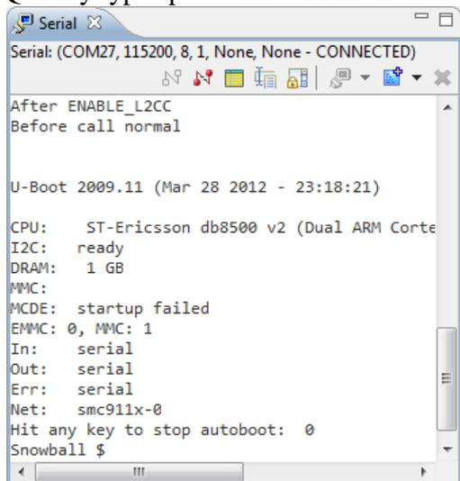
If nothing happens, try disconnecting and reconnecting the target power again. When you remove power from the Snowball, the serial connection will be broken and the Serial view will begin repeating **Bad file descriptor in nativeavailable**. Click the Disconnect button (🔌) in the **Serial** view, reconnect the power (without pressing the power button) and then click the Connect button (🔌).
