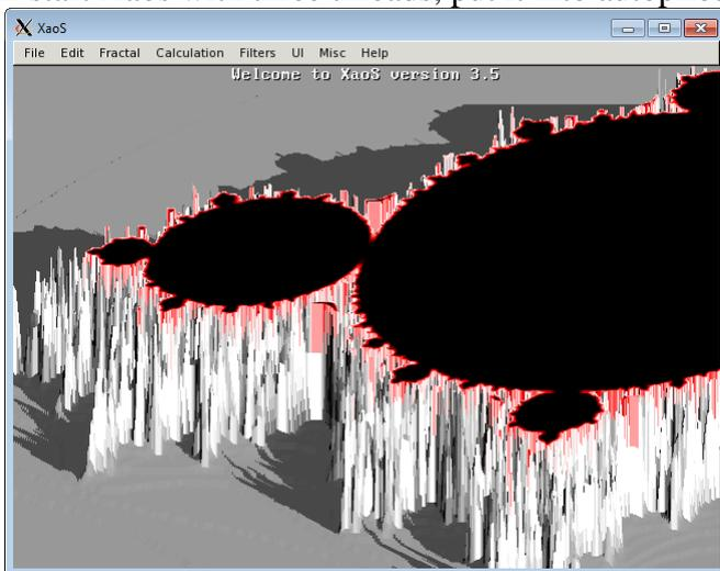
You can also set the options from the Xaos GUI by selecting **UI > Autopilot** and **Filters > Pseudo 3d**. (When running with multiple threads the Xaos program has some display glitches and even hangs sometimes, but it's still useful as a demonstration. You can quit it and start it over if it gets stuck.)
