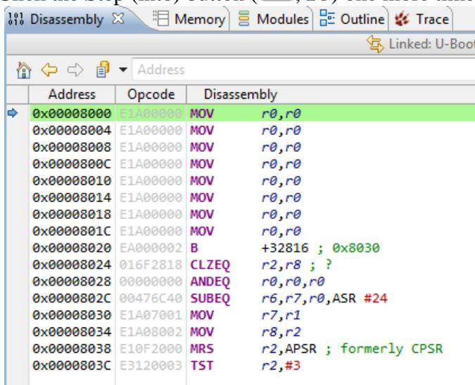
The kernel image that U-Boot loads into RAM is known as **uImage**. It has a 64 byte header created by the U-Boot tool `mkimage` and is followed by a compressed version of the kernel wrapped by a self-decompressor which is the code we see here and is known as a **zImage**. The **zImage** works by decompressing the kernel code in-place and then jumping back to the beginning again. We'll set a **hardware** breakpoint on the first instruction and continue the target to let the decompression happen.
