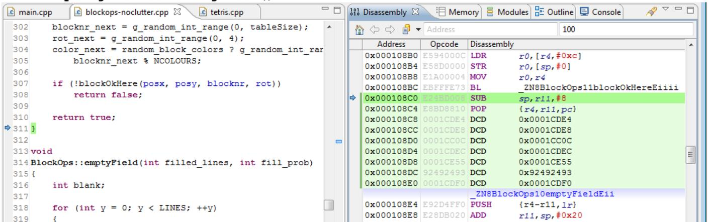
The `BlockOps::blockOkHere()` frame is gone from the call stack. Since the return value from a function is in register R0, we can use the **Registers** view to see that `BlockOps::blockOkHere()` has returned a value of `true` (1) which is also the value that `BlockOps::generateFallingBlock()` is going to return.
