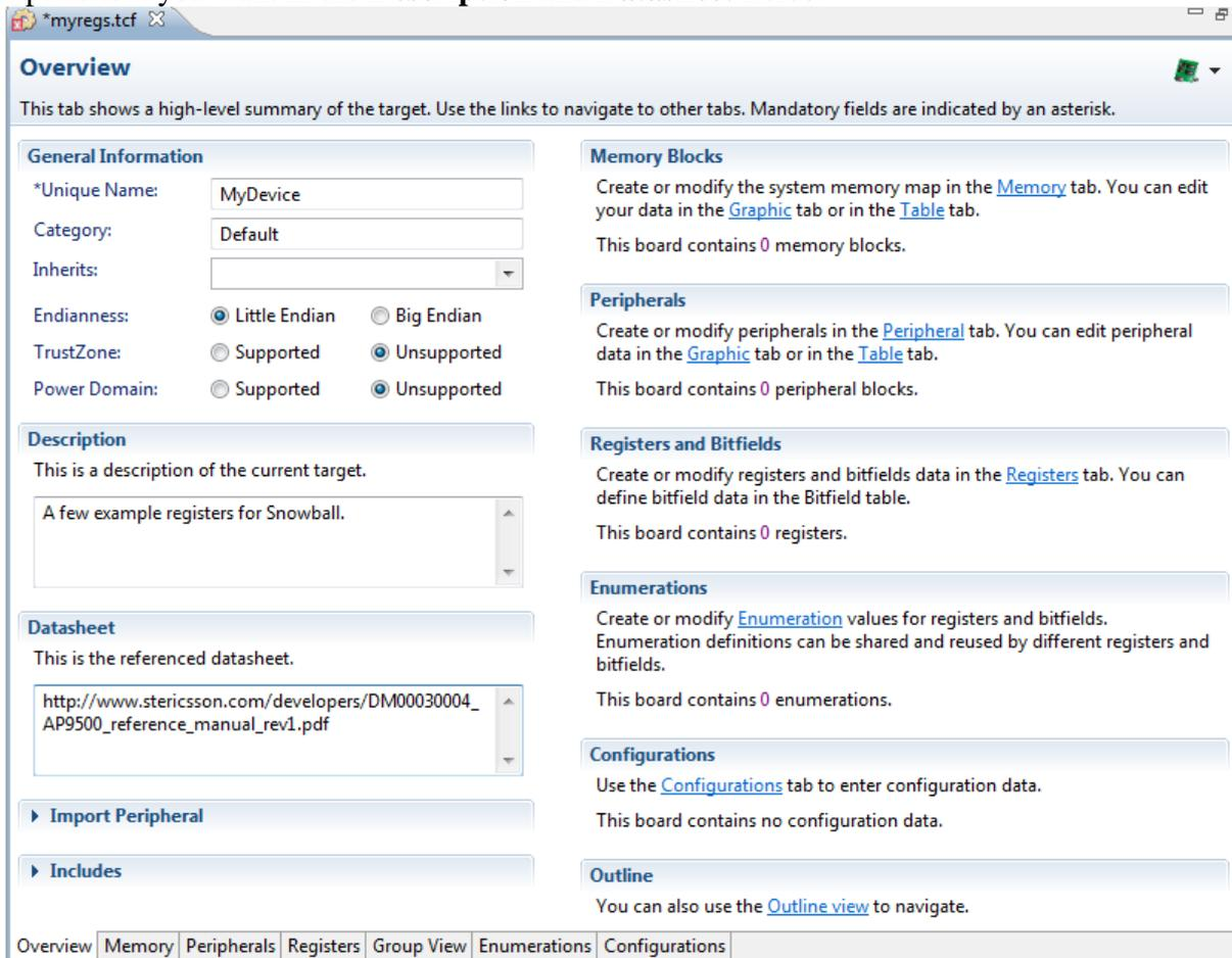
The **Target Configuration Editor** has a number of panes which are used to describe various aspects of the target: **Memory**, **Peripherals**, **Register**, **Enumerations**, **Group View** and **Configurations**. They are described on the right side of the **Overview** pane along with links. There are also tabs along the bottom of the view for switching panes. You can also navigate a **.tcf** file using the standard Eclipse **Outline** view.
