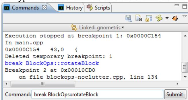
You can use a function name, a file name and line number (for example, **blockops-noclutter.cpp:134**) or an address (for example, **\*0x11690**) as the argument to the **break** command.
