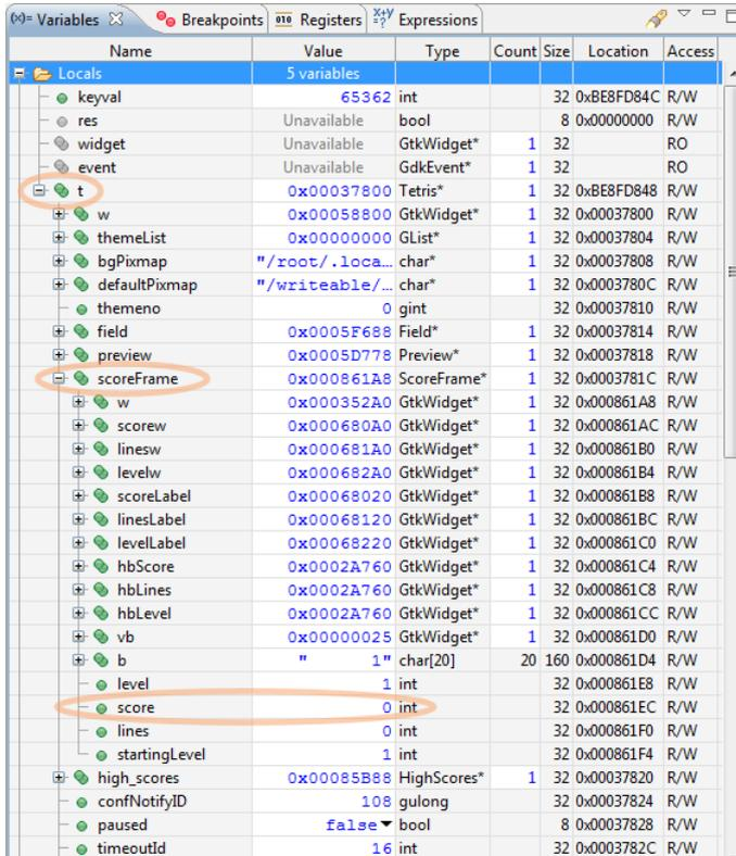
⇒ Click on the `score` value and type a new value. The new score will not show up on the Gnometrus display immediately. It will be displayed the next time the score is redrawn. (The changes to the Gnometrus code mentioned earlier cause the score to be redrawn every time a block moves down.)
