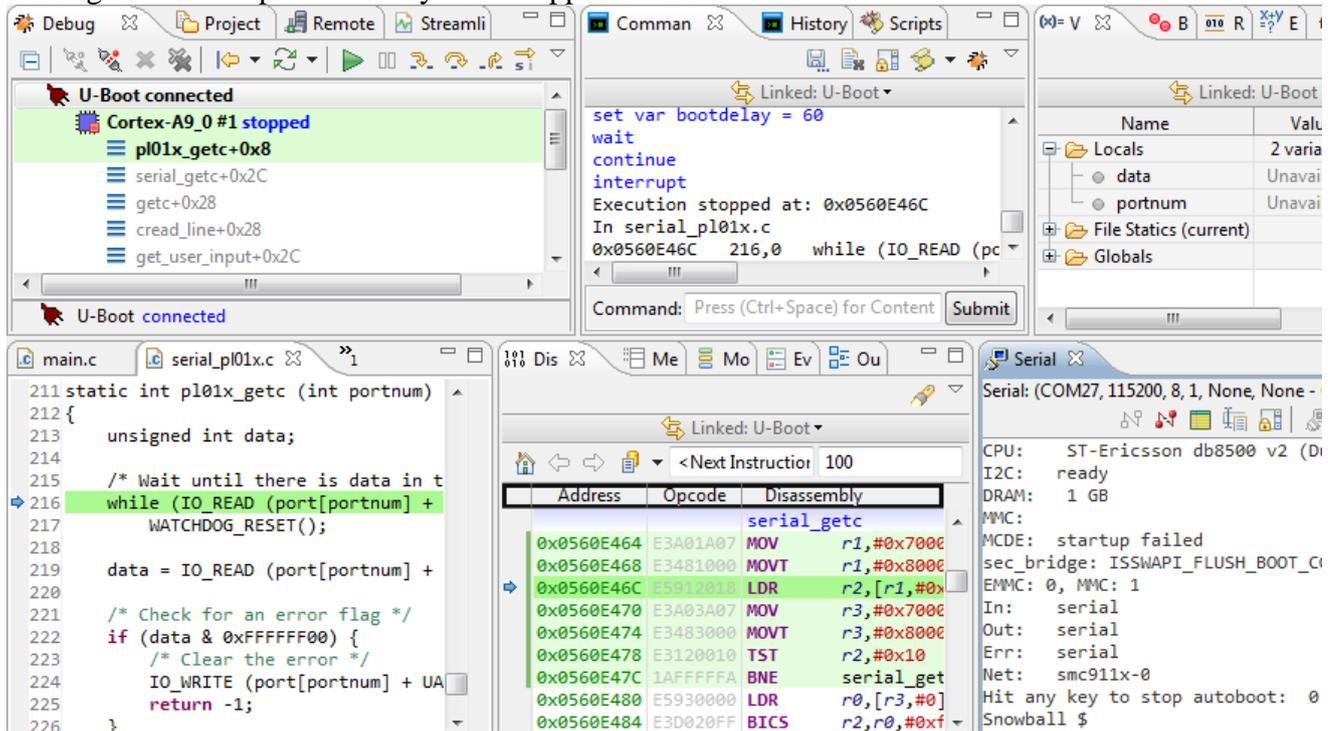
[If you see no functions in the stack and the `PC` is at an address like `0xC00xxxxx` then you have not stopped in U-Boot and the kernel has booted. Reset the target (power off and on) and stop U-Boot from booting the kernel by typing to the **Serial** view.]
