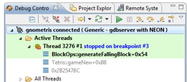
Stepping can happen either by source line or assembly instruction. The **Debug Control** view has a toggle button (⏪; ⏩) that you can use to switch between the two modes. By default stepping is by source line with the 's' dark (⏪).
