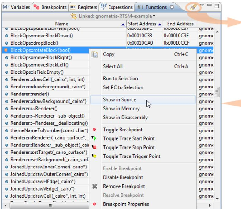
⇒ Double click on `BlockOps::rotateBlock()` to set a breakpoint on it. The breakpoint symbol (●) will appear. Then right-click on `BlockOps::rotateBlock()`; then choose **Show in Source** from the context menu.
