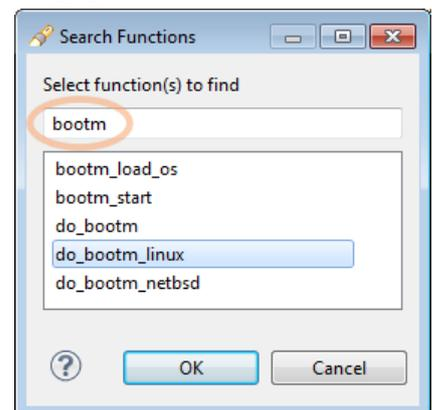
The entry for `do_bootm_linux` is selected. We can set a hardware breakpoint on it even while the target is running.
