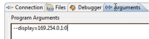
The `--display=169.254.0.1:0` argument tells Gnetris to open its window on the X server running on the host. If you want Gnetris to display on the target's own X server, you would use `--display=:0` instead.
