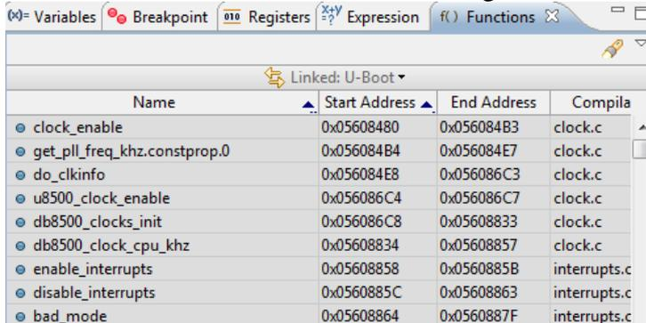
The **Functions** view shows information about all of the functions in the debug symbols we have loaded including the start and end addresses. You can change the sorting of the **Functions** view by clicking on the column headings. You can use the **Filters...** command in the view's drop-down menu (▼) to control which images and compilation units are shown.
