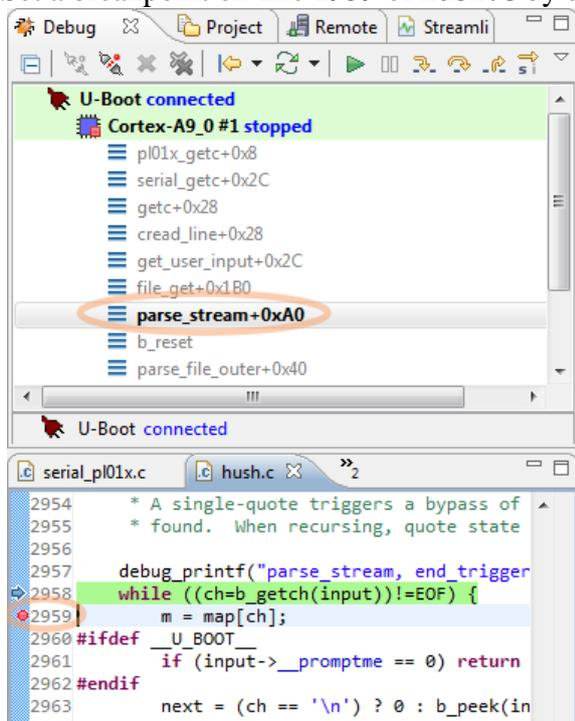
You can see the breakpoint (●) appears in both the source and **Disassembly** views. The breakpoint is also listed in the **Breakpoints** view where it's possible to set conditions and other fancy stuff that we see later.
