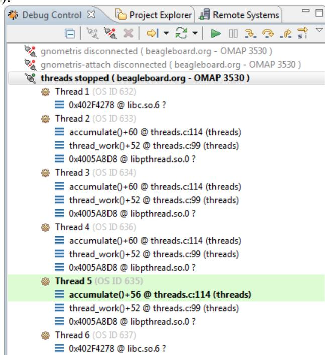
Below each thread will be the frames of its call stack. You can change the debugger's focus from one thread to another by clicking on the different threads. You can collapse all of the threads by clicking the Collapse All button (
