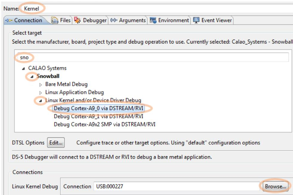
We'll leave the **Files** pane of the debug configuration blank so that we can be sure that the target is stopped when we load the debug symbols. We'll load them in a script in the **Debugger** pane. The kernel was (and can only be) built on a Linux host. As we are using a Ubuntu image we can use the Linux package manager to get the symbols for the Linux kernel.
