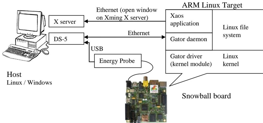
The kernel driver (called `gator.ko`) together with a daemon running on the target (called `gatord`) captures the data and sends it over the network to the host PC for analysis. The kernel module must be built against the Linux kernel in use on the target.
