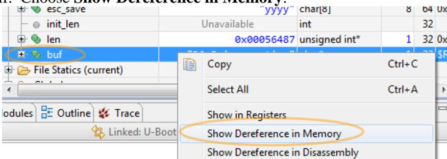
The memory that `buff` is pointing to is displayed in a **Memory** view. Because it's not possible in C to know how many bytes `buff` is pointing at, only one byte is shown.
