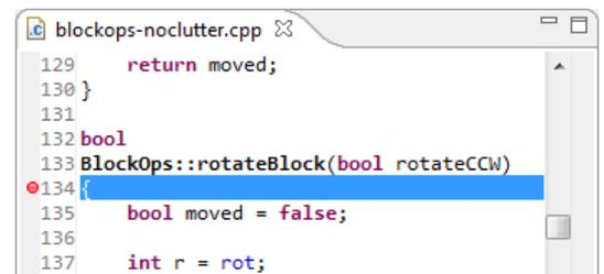
We can see that the breakpoint we've set is on line 134 of `blockops-noclutter.cpp`. We could also use the **Project Explorer** view to open the source file `blockops-noclutter.cpp` by double-clicking on it.
