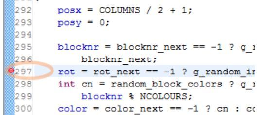
You can also set a breakpoint by double-clicking in the left margin of a source or disassembly line where the breakpoint symbol ( ● ) will appear. You can delete a breakpoint by double-clicking it, too.
