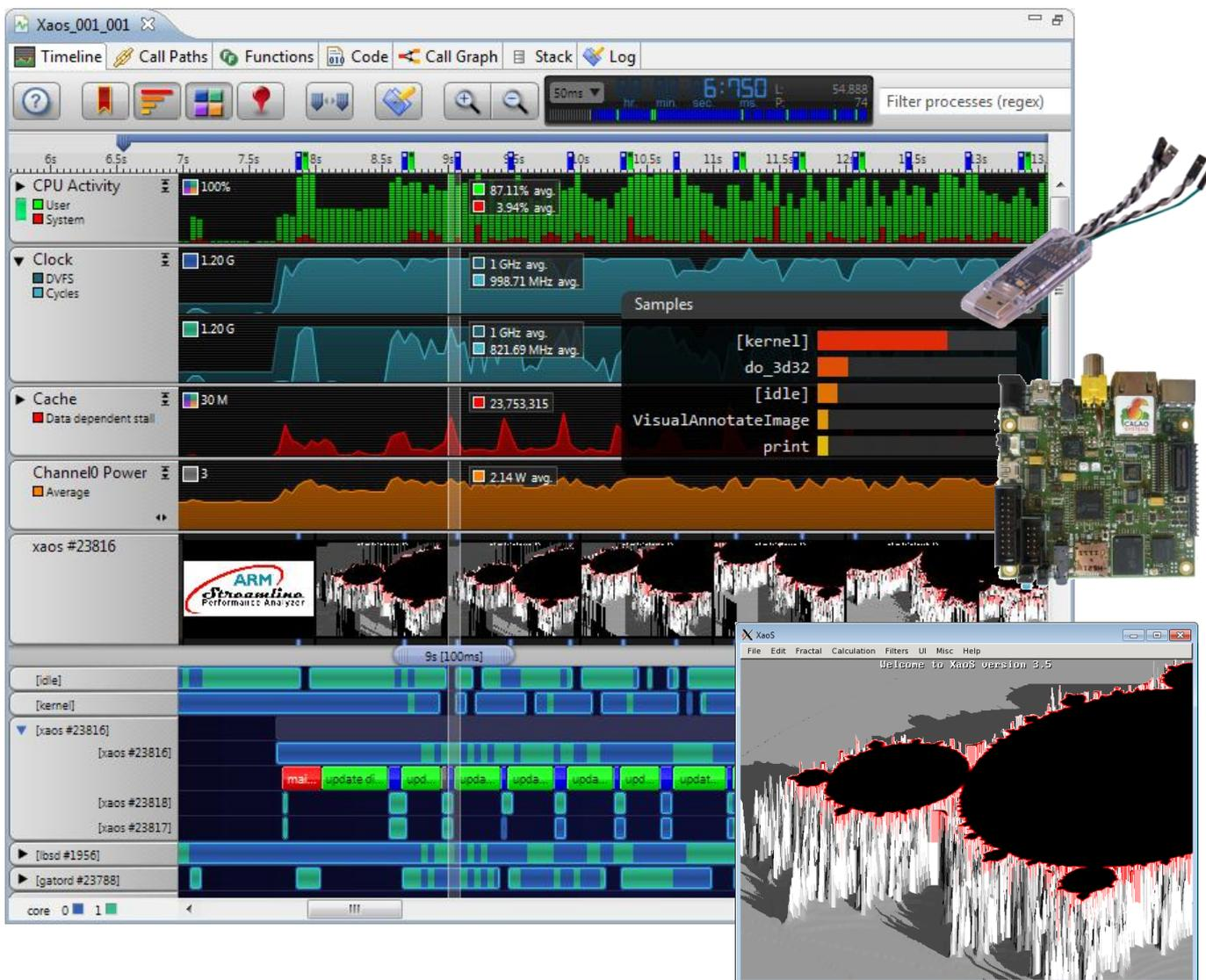
ARM® Streamline™ is a graphical performance analysis tool. Combining a Linux kernel driver, target daemon, and an Eclipse-based user interface, it transforms sampled data and system trace into reports that present the data in both visual and statistical forms. ARM Streamline uses hardware performance counters along with kernel metrics to provide an accurate representation of system resource use.
