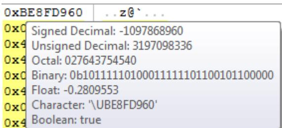
You can toggle these tooltips off or on with the **Show Tooltips** command in the **Memory** view's drop-down menu (▼).
