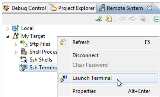
This will open a **Terminals** view in Eclipse that can be used to execute commands on the target. (This is different from, but confusingly similar to the **Serial** view).
