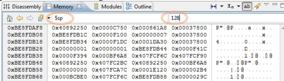
The memory address of the first byte in each row is displayed in the left margin. The width of the view determines how many bytes are displayed on each row.
