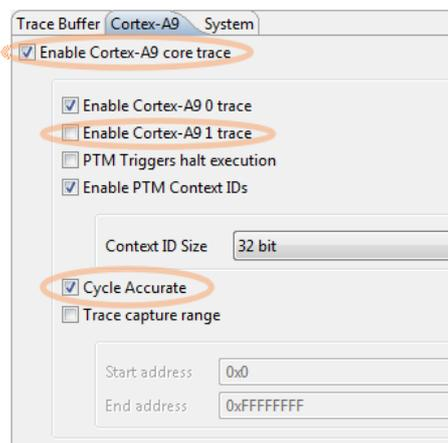
You can leave **Enable PTM Context IDs** checked. U-Boot doesn't change the context ID so how we set it won't matter. You can disable **Cycle Accurate** trace if you want more instructions to fit into the ETB. It's also possible to setup an initial trace capture range to limit what instruction addresses are captured, but we don't want to do that.
