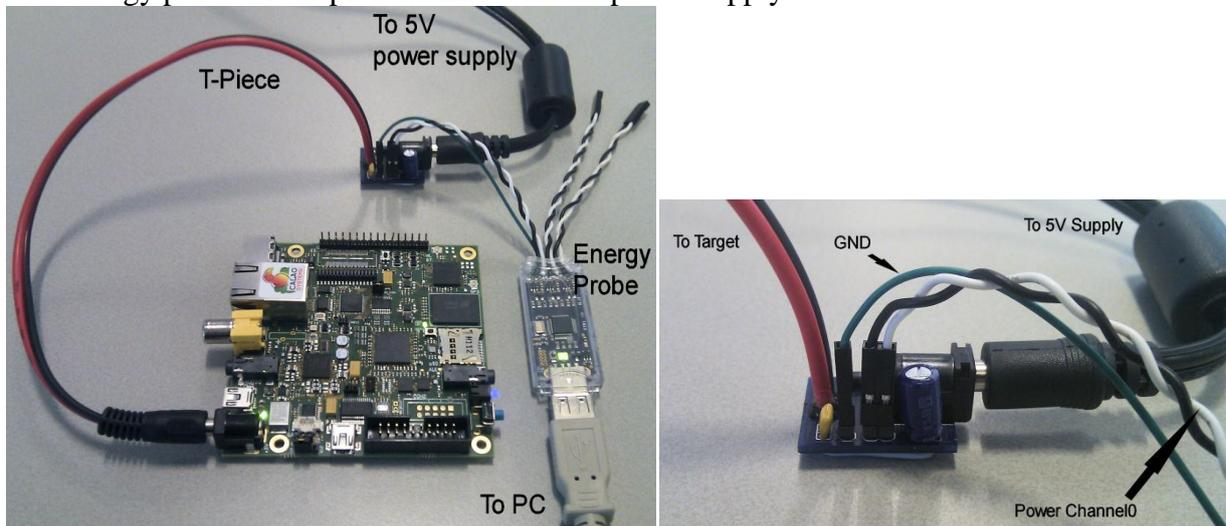
When you first connect the probe to your PC you will need to install a driver from the DS-5 installation. On windows this is typically `c:\Program Files\DS-5\sw\energy_probe`. Once the driver is installed, the probe connected and the target powered on the Energy Probe will display a green LED.
