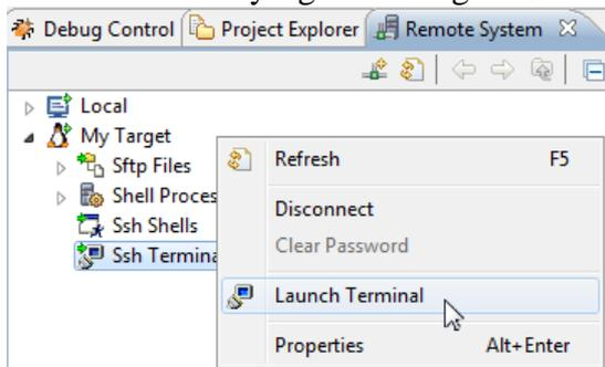
This will open a **Terminals** view in Eclipse that can be used to execute commands on the target. (This is different from, but confusingly similar to the **Serial** view). The picture below shows the output from the example target image included with DS-5. If your target is running a different distribution the output will be different.
