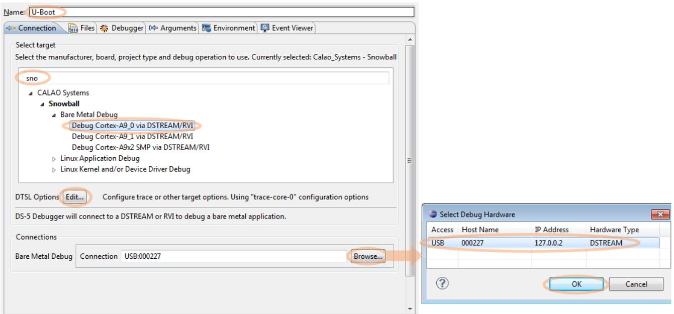
The tracing options are configured in a separate DTSL configuration. “DTSL” stands for Debug and Trace Services Layer. We’ll enable tracing on core 0.
