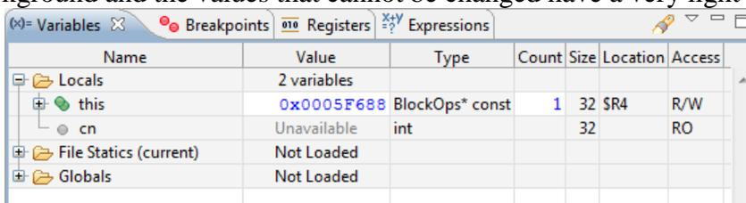
The **Locals** part of the view shows the arguments and local variables to the function. Because of the current location of the PC the variable `cn` is not available yet. We will be able to see it after we have stepped past its initialization on line 298. Since `BlocksOps::generateFallingBlock()` is a C++ member function it has a `this` argument that is a pointer to a `BlocksOps` structure.
